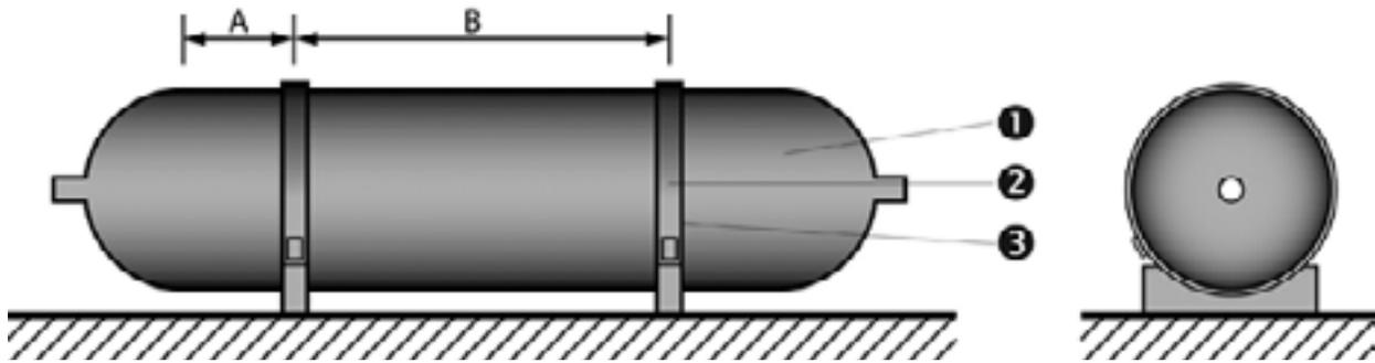
Minimum dimensions: A = 25mm (0.984”), B = 1/3 of cylinder length
