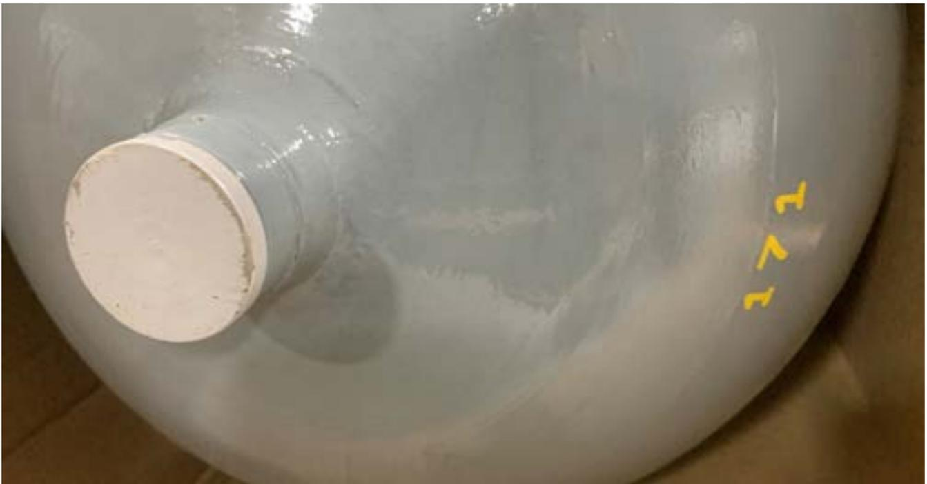
Sample of a cylinder serial number on each WireTough cylinder.
