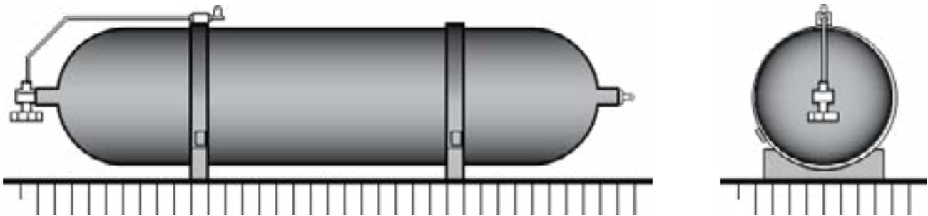
Shared PRDs - Some fuel systems can have multiple cylinders plumbed to a single PRD or set of PRDs; these are generally plumbed either from end plugs of multiple cylinders or from valves of multiple cylinders. Contact WireTough for more information about approved configurations for shared PRDs.
