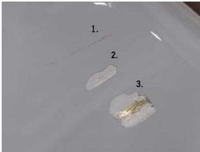
Cylinder surface is comprised of an under layer of epoxy and an outer layer of polymer.
