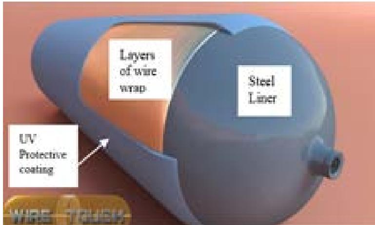
WireTough Cylinders, LLC produces pressure vessels for storing CNG, breathing air, and hydrogen at pressures ranging from 250 to 875 bar (3,600 to 13,000 psi). At these pressures, WireTough's products have distinct advantages because they offer longer service life and higher durability at very competitive prices. WireTough has designated their cylinders as Type II-S to differentiate them from Type II cylinders wrapped with fiberglass or carbon fiber.
