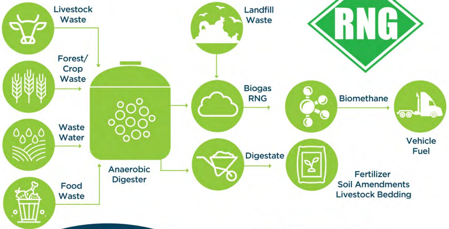
**Renewable Natural Gas (RNG)**, or biogas, is gas produced from methane emitted through the decomposition of animal manure, food waste, forest management waste, wastewater sludge, and garbage.
