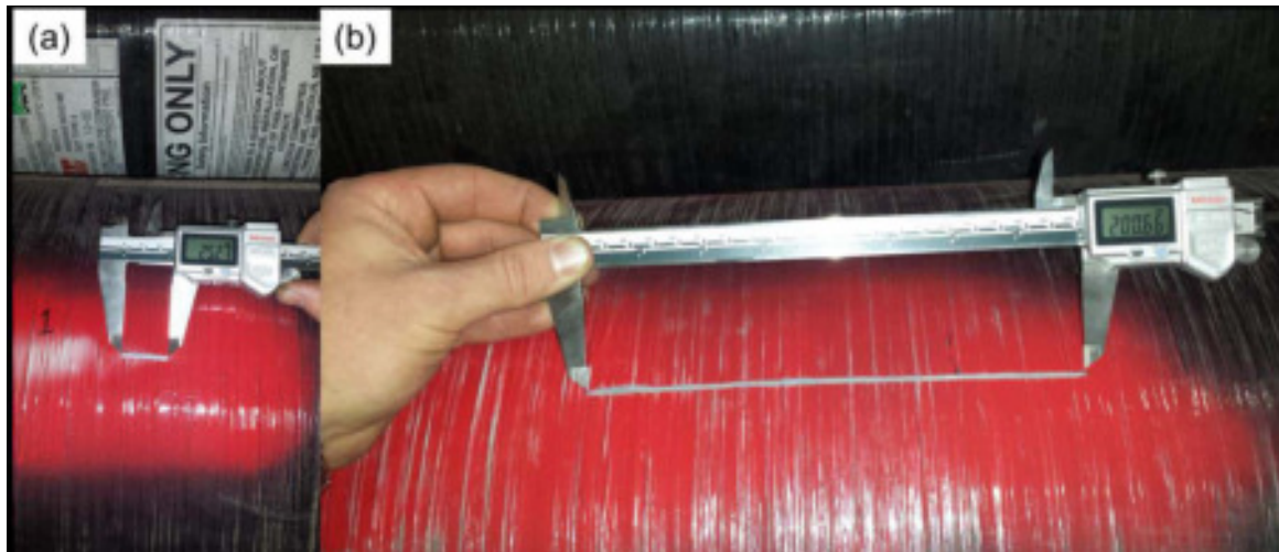
Figure 3. (a) Representative short notch with deep depth and (b) representative long notch with shallow depth
