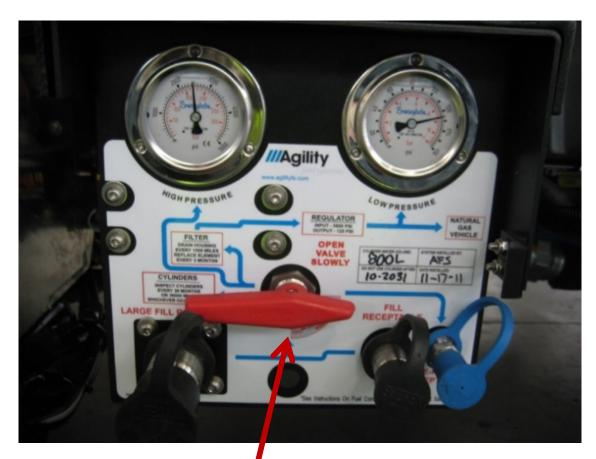
Fuel System Isolation Valve (manual valve, ¼ turn valve)
